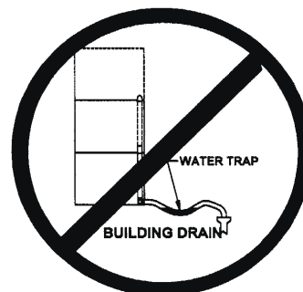
IMPROPER DRAIN LINE CONNECTION
